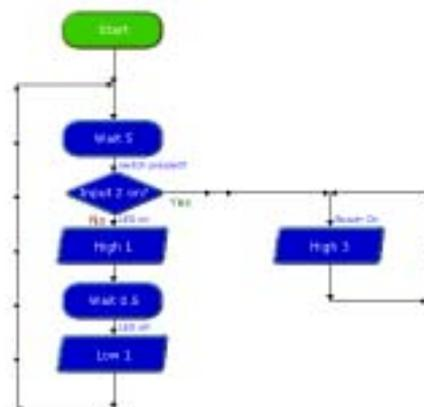
The student's first attempt at programming is shown in flowchart 1 above. This is the obvious solution, but does not work as expected. This is because the alarm does not sound immediately when the wire is cut - as the input is only checked once every 5 second there can be up to 5 seconds 'lag' before the alarm sounds.
