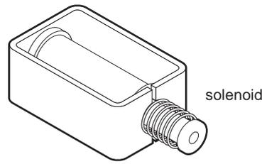
A solenoid consists of a steel plunger inside an electric coil which is wrapped around a tube. When the coil is energised a magnetic field is created, and this draws the plunger into the tube. When the coil is de-energised a spring pushes the plunger back out of the tube.
