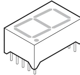
A better solution is to use a dedicated integrated circuit, such as the CMOS 4511B to control the seven segment display. This IC controls the seven segment display according to the binary 'code' on the four data lines. This system uses four pins rather than 7.
