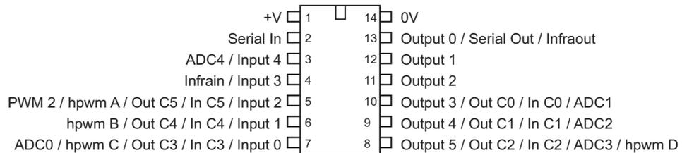
The PICAXE-14M is a very versatile device. In its default state, which is designed primarily for educational use, it has a simple, clean 'inputs on left' - 'outputs on right' layout.
