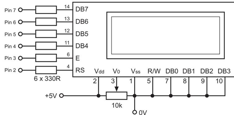
Before the sub-procedures are studied, it is important to understand how the LCD module operates. It has two modes of operation, which are called 'character' mode and 'instruction' mode. The RS pin (pin 2) controls the mode - when high the LCD is in character mode, when low the LCD is in instruction mode.
