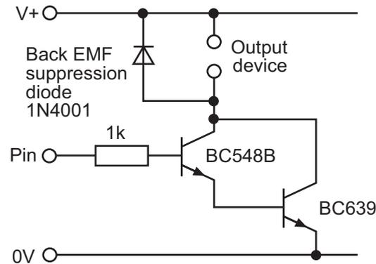
However this circuit requires that two separate transistors are used. It is possible to buy a device that contains the two transistors in a single package. This transistor is called the BCX38C, and can switch currents up to 800mA. This is the transistor used in all the circuits through this book.
