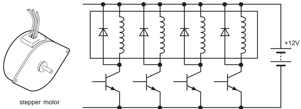
As the stepper motor operates at 12V, the standard transistor circuit is required to switch each coil. As the coils create a back emf when switched off, a suppression diode on each coil is also required. The table below show the four different steps required to make the motor turn.
