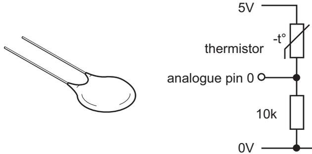
It should be remembered that the thermistor response is not linear, and so the readings will not change in exactly the same way as with a potentiometer. In general there is a larger resistance change at lower temperatures. This can be compensated for in the software by using a smaller range at higher temperatures. Experiment to find the most appropriate settings for the circuit.
