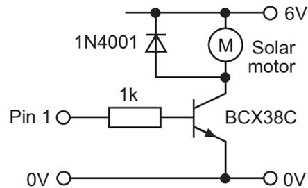
This circuit uses a darlington transistor to switch the motor on and off. This circuit will work with 'solar' motors, but may not function correctly with cheap dc 'toy' motors. This is because this type of motor introduces a lot of electrical 'noise' on to the power rails. This noise can affect the microcontroller, and in some cases can completely stop the control program functioning.
