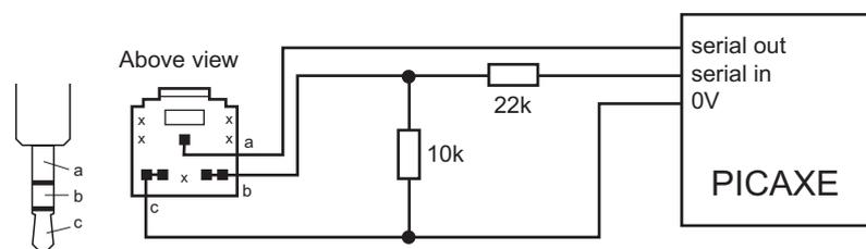
Note that the two resistors are not a potential divider. The 22k resistor works with the internal microcontroller diodes to clamp the serial voltage to the PICAXE supply voltage and to limit the download current to an acceptable limit. The 10k resistor stops the serial input 'floating' whilst the download cable is not connected. This is essential for reliable operation.
