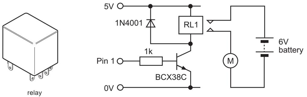
The above circuit will only switch the motor on and off. If the motor is required to run in both directions (forwards and reverse), two relays can be used as shown.
