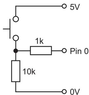
With this circuit the input pin is **high** when the switch is open and **low** when the switch is closed.
