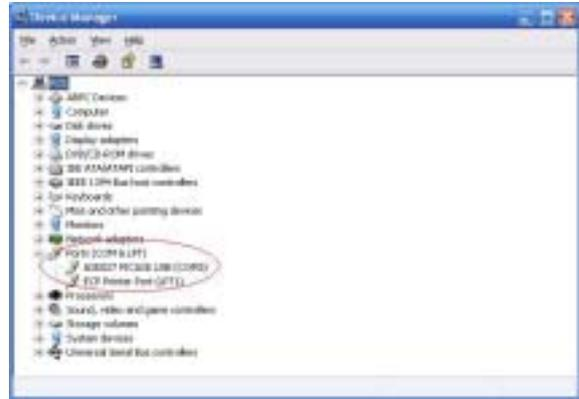
The Device Manager will then start - click the '+' symbol beside 'Ports (COM & LPT)' so that all the entries are visible. Beside the 'AXE027 PICAXE USB' entry will be the currently allocated COM port number. The instructions given later in this manual explains how to change this COM port number if necessary.
