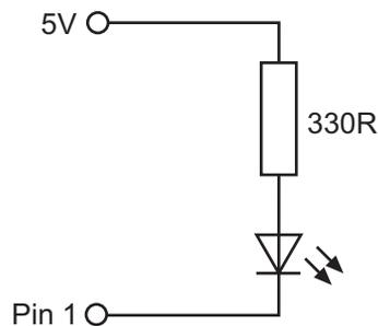
Bi-colour LEDs often contain both green and red LEDs connected in ‘inverse parallel’. This means if current flows one way through the device the LED lights green, and if current flows the other way the LED lights red. Therefore by using the sink/source capabilities of the PICAXE microcontroller it is possible to light the LED in both colours.
