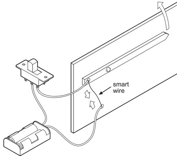
Shape Memory Alloy wire or springs are 'smart' materials that can be used to create mechanical actuation (movement). When an electric current is passed through the wire it heats up and so contracts with a large pulling force. When the current is removed the wire cools and so expands again (a 'traditional' steel spring is sometimes used to pull the smart wire/spring taut as it cools).
