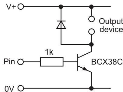
Note that it is usual to connect a back emf suppression diode across the output device. This is essential with devices such as relays, solenoids and motors which create a back emf when power is switched off. The diode type 1N4001 is the device recommended.
