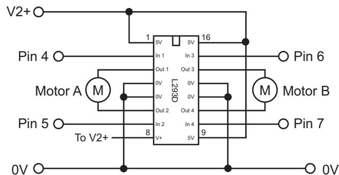
Four pins from the microcontroller are connected to the four transistor 'pairs' via IC pins 2, 7, 10 and 15.
