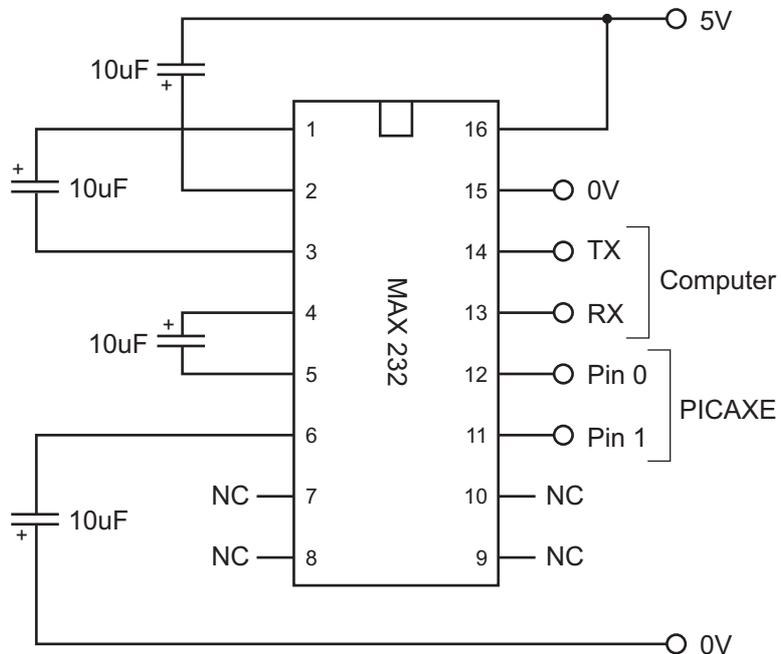
NB. Note polarity - capacitors connected to pins 2 and 6 are connected 'upside down'.
