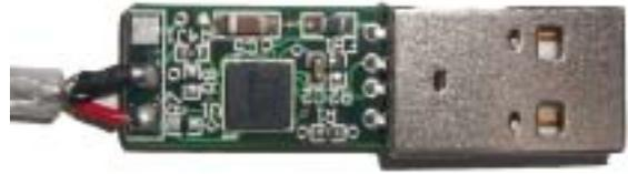
However, as many different products from many different companies all use the same FTDI chip, each product is given a unique 'product id' number for identification purposes. This unique product id is programmed into the chip inside the cable, so that when the cable is connected to the computer it can be uniquely identified.
