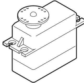
A typical servo has just three connection wires, normally red, black and white (or yellow). The red wire is the 5V supply, the black wire is the 0V supply, and the white (or yellow) wire is for the positioning signal.
