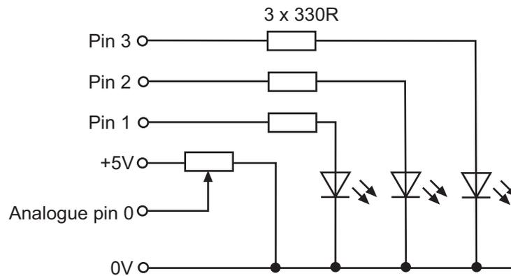
The program below lights three different LEDs (connected to pins 1, 2 and 3), depending on the analogue sensor reading.
