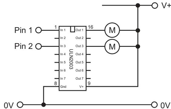
A device called the ULN2803 Darlington Driver IC is also available. This is identical to the ULN2003 except that it is an 18 pin device and contains 8 darlington pairs instead of 7. If it is necessary to pass relatively high currents through a device it can be useful to 'pair up' drivers as shown with this circuit.
