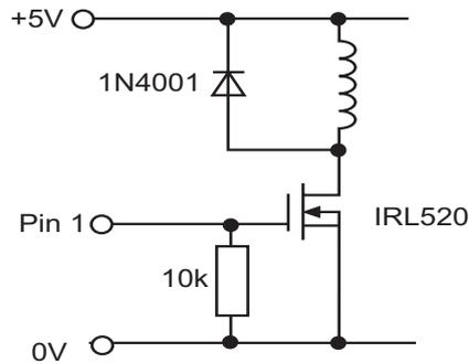
The isonic solenoid valve can be used to control air flow through a pneumatic system. Isonic valves are ideal for battery operated products as operate at a low voltage and draw much less current than traditional solenoid valves. The standard transistor switching circuit can be used to drive the isonic valve.
