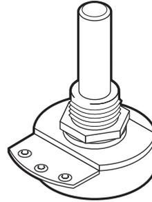
The readADC command is used to measure the value of the resistance by carrying out an Analogue to Digital Conversion. The value of the resistance is given a 'value' between 0 and 255 which is then stored in a variable. After storing the reading in the variable, the if...then command can be used to perform different functions.
