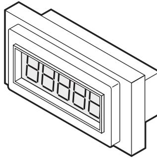
The Counter Module is a numeric LCD display module that can be used to show a 'counter' value. To increment the counter a pulse (between 1 and 1.5V) must be applied to the counter pad 3. As the PICAXE microcontroller operates at 5V a potential divider formed from resistors must be used to reduce the PICAXE microcontroller output signal to 1.5V. As the counter uses it's own, internal, 1.5V battery, the two 0V rails must also be connected.
