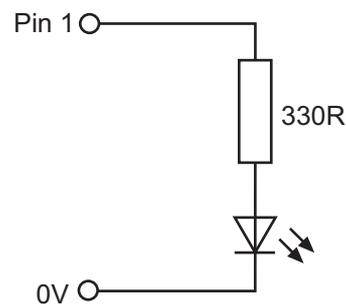
LED connected to Power Rail.
