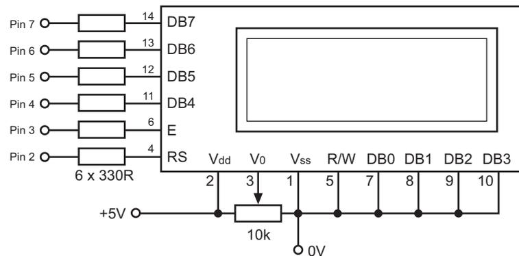
The LCD has 6 lines that can be connected directly to the PICAXE microcontroller pins. However it is a good design practice to add a low value resistor (e.g. 330R) on the lines to protect against static discharges. The 10k potentiometer connected to pin 3 is used to adjust the contrast of the display. All unused lines should be tied to ground as shown.
