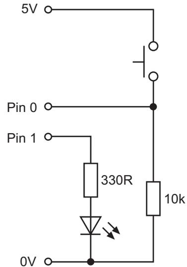
The following two programs show the effect of switch bouncing. The program should light the LED on pin1 when the switch connected to pin0 has been pressed more than 5 times. However, the first listing may not work correctly, because the microcontroller may count 'bounces' rather than actual pushes, and so the LED may light prematurely.
