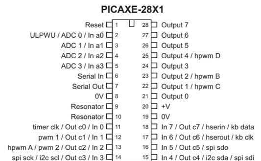
This gives a maximum of 12 digital inputs, 16 outputs and 4 analogue inputs
