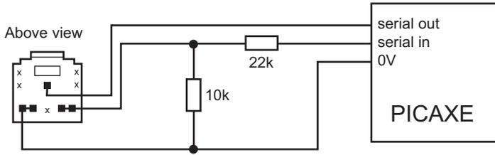
The standard PICAXE download socket (part CON039) and 10k/22k download circuit is unchanged for use with the AXE027 USB cable (ie the same circuit is used for both the AXE026 serial cable and the AXE027 USB cable).
