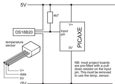
This program uses the readtemp command to read the temperature from a DS18B20 digital temperature sensor connected to input 1.
