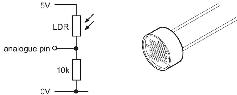
It should be remembered that the LDR response is not linear, and so the readings will not change in exactly the same way as with a potentiometer. In general there is a larger resistance change at brighter light levels. This can be compensated for in the software by using a smaller range at darker light levels. Experiment to find the most appropriate settings for the circuit.
