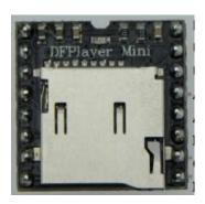
The SPE035 PCB was primarily designed to be used with a 'DF Player Mini' (or fully compatible clone such as BY-TF-16P). This is the recommended module and is used in position 'A'.
