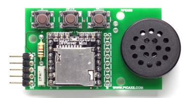
The SPE035 Serial MP3 player consists of a small MP3 player module mounted on a PCB with serial connector, test switches and 8 ohm speaker. It provides a simple and low cost way to add MP3 tune playback to any PICAXE project.
