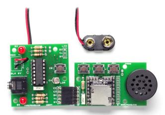
To use the SPE035 it is first necessary to issue the 'initialise' command to the module (this tells the module to read files from the microSD card). Depending on the quantity of MP3 files this can take up to 4 seconds, but may be much quicker. The play command is then used to play the desired tune (0001.mp3).
