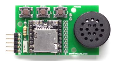
Note that there are two positions (A or B) on the PCB for the MP3 player module. This is because MP3 playback modules using the YX5300 MP3 chip are available in various different types and sizes. Carefully check the position of your module before soldering on to the board.
