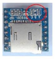
The PCB is also compatible with the 'BY8001-16P' module. This is used in position 'B' as it has a different size/pinout. Note that for serial control of the BY8001 it **must** be put into 'serial mode 111' by **removing all 3** resistors shown in the red circle (the default is normally a resistor in positions 'A' and 'C' with 'B' already removed).
