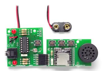
The following examples assume use of the AXE171 PICAXE 14 Audio Kit, so if using a different board you may need to alter the input / output pins in these examples (which are 'serial transmit' on output B.4 and 'busy signal' receive on input pinC.2).
