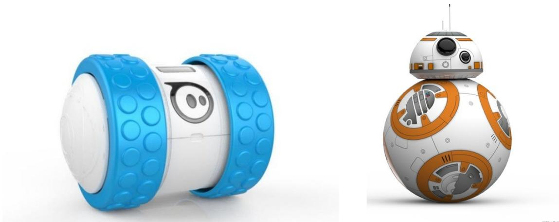
*The Ollie and BB8 robots both use an identical bluetooth low energy communication protocol and have the same features, so are regarded as being the 'same' robot via S2Bot.*
