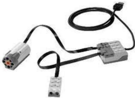
The WeDo 1.0 connects to the computer via a USB cable. There are no drivers to install on Windows or Mac, so WeDo should work straight away. For Linux please see the appendix.
