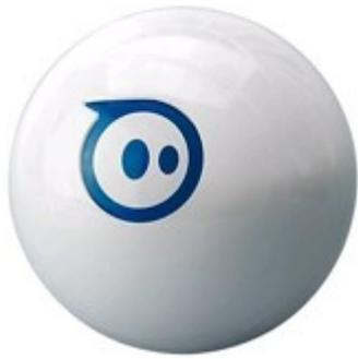
The Sphero can be changed colour or moved in various directions at various speeds. The direction is always relative to the current 'heading'. The only way to see the current heading is to switch the blue tail light on, the current heading (0 degrees) is then directly opposite the tail light position.
