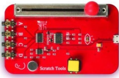
The PicoBoard normally has a USB connector and connects to the computer via a USB cable. Installation of the USB driver is described in the appendix at the end of this document.
