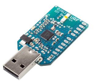
The URF is the easiest and most convenient way to wirelessly communicate between a PICAXE chip and a computer. Simply connect the URF directly to the USB port of your computer and an ERF module to the PICAXE chip.
