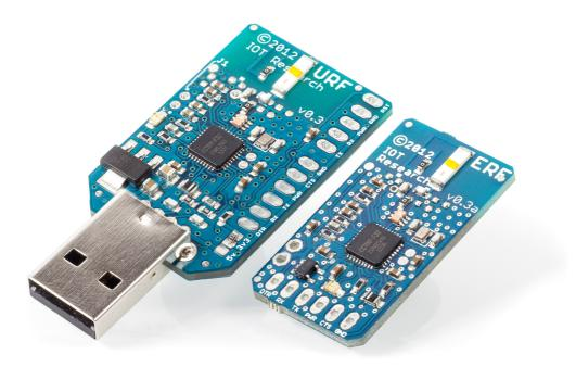
The ERF, URF and XRF modules are designed to provide 'out-of-the-box' instant wireless bidirectional serial communication between a computer and/or multiple PICAXE project boards. All 3 modules are designed around the Texas Instruments CC111x combined micro & RF transceiver integrated circuit.
