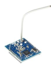
The XRF is an XBee footprint compatible module to allow wirelessly communication between a PICAXE chip and a computer, or between 2 (or more) PICAXE chips. The XRF transparently passes serial characters to and from individual or multiple radio devices. You don't need to use complex encoding or error checking as it is all done for you - simply send raw text/data via 'serout', and receive text/data via 'serin'.
