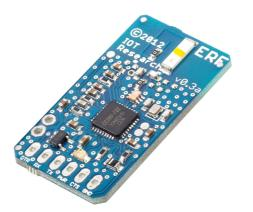
The ERF is the easiest and most convenient way to wirelessly communicate between a PICAXE chip and a computer, or between 2 (or more) PICAXE chips.
