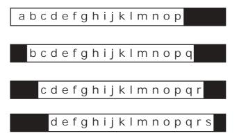
On most LCD displays there is memory for 40 characters on each line. Each space in the RAM memory can be thought of as a 'box' which is ready to hold a single character. Each RAM 'box' has a numbered address to describe it. The first line RAM 'boxes' are at addresses 128 to 191, the second line RAM 'boxes' are from 192 to 255.
