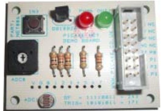
Assembly of the demo board is very straight forward (soldering experience is assumed).
