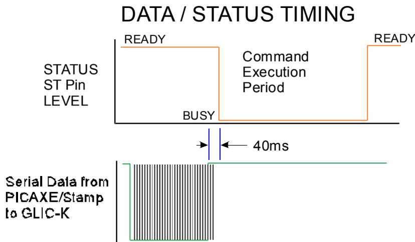
This diagram shows the STATUS pin level after valid data has been sent to GLIC-K1.
