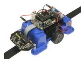
Note - ensure you connect the cable to the inner CABLE holes on the microrobot PCB (not the outer SRF005 connection holes!)
