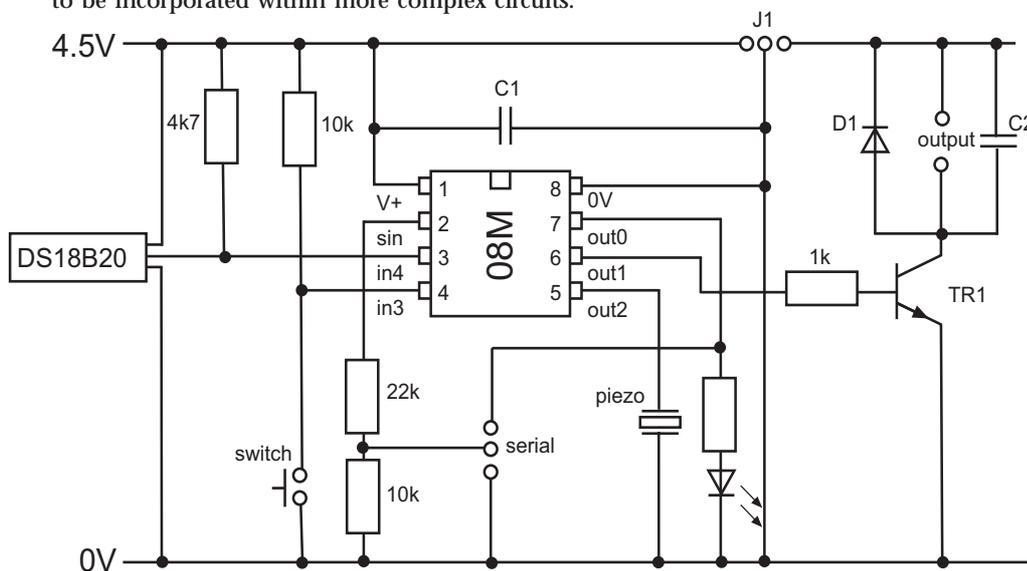
The circuit is based around an 8 pin microcontroller, the low-cost PICAXE-08M.
