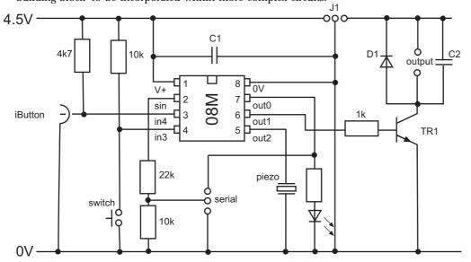
The circuit is based around an 8 pin microcontroller, the low-cost PICAXE-08M. The circuit is fairly self-explanatory and includes the following features:
