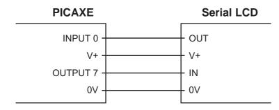
Note: The connections must be made directly to the PICAXE output pins (not via the darlington driver buffered outputs found on the PICAXE starter pack project boards)
