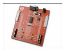
To upgrade the system simply remove the old 18 pin chip in the centre of the Stamp Controller and replace with the new PICAXE-18M2-ST chip, ensuring pin1 is at the top of the board. That's it – easy to do in under 30 seconds!
