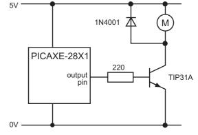
Motor driver circuit - repeated on each output
