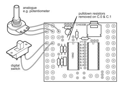
The connections marked C.3 and C.4 should not generally be used with the PICAXE system. These are used by the PICAXE chip as the 'serial in' and 'serial out' PC download connection.
