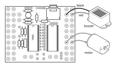
Note that motors should be suppressed by soldering a 220nF polyester capacitor (part CAP002) across the motor terminals to prevent electrical noise affecting the circuit.
