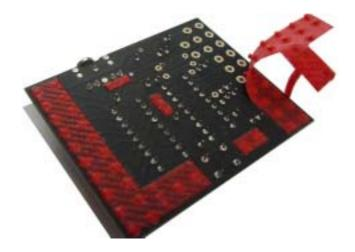
This peelable layer protects the user solderable pads during manufacture and storage, to keep the pads clean and grease free.
