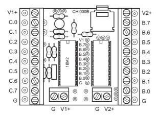
Note that when using terminal blocks it is necessary to 'share' the V2+ connector with all output pins and to 'share' the V1+ connector with all inputs. Remember that with the darlington driver output buffer the output devices are connected between V2+ and the output (NOT output to 0V). Like wise the inputs are connected between V1+ and the input.
