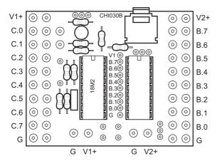
To use the board with an older (now discontinued) 18/18A/18M/18X PICAXE part an extra 1k resistor \*MUST\* be soldered to the board in the 'RST' resistor position. If desired an optional reset switch (part SEN030) may also be fitted in position 'S1'. Note that the current release PICAXE-18M2 does not have a reset pin, so does not require the RST resistor or the reset switch to be fitted.
