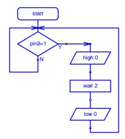
The LED on output 0 should light whenever the switch is pushed. If it does not check that the switch and 10k resistors are correctly soldered.
