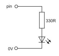
The value of the resistor required depends on the battery voltage used. For a 4.5V battery pack a 330R resistor can be used, and for a 3V battery pack a 120R resistor is appropriate.
