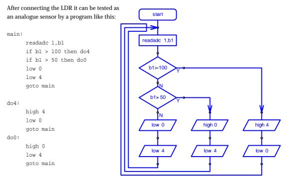
The 'readadc' command is used to read the analogue value (a number between 0 and 255) into variable b1. Once the number is in variable b1 it can be tested to see if it is greater than 100 or greater than 50. If it is greater than 100 output 4 is switched on, if it is between 50 and 100 output 0 is switched on, and if it is less than 50 both outputs are switched off.
