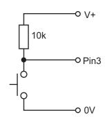
This layout is a little confusing, as it means that when the switch is pushed down, the logic level is '0'. When the switch is not pushed the logic level is '1'. This is known as an 'active-low' switch. In this project this is necessary for compatability with the optional infra-red upgrade kit.
