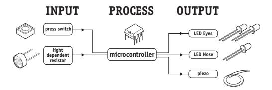
The electronic block diagram is shown below. output - pin0 and pin4 are connected to the LEDs output - pin2 is connected to the piezo sounder input - pin1 is connected to the LDR input - pin3 is connected to the push switch
