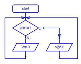
This program will switch output 0 on and off according to the light level.
