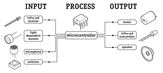
The electronic system that controls the Furby toy can be drawn as a 'block diagram'. The light sensor, microphone and switches all provide information to the microcontroller, and so these are known as 'inputs'. The microcontroller then 'decides' how to behave and may then operate the outputs e.g. make the motor move or generate a sound with the speaker. If another Furby is nearby they can 'communicate' by infra-red signals transmitted, and received, by the microcontroller.
