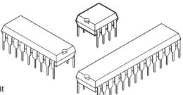
The microcontroller is an integrated circuit ("chip") that contains memory (to store the program), a processor (to process and carry out the program) and input/ output pins (to connect switches, sensors and output devices like motors).
