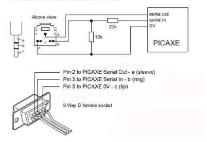
Note that the two resistors are not a potential divider. The 22k resistor works with the internal microcontroller diodes to clamp the serial voltage to the PICAXE supply voltage and to limit the download current to an acceptable limit. The 10k resistor stops the serial input 'floating' whilst the download cable is not connected. This is essential for reliable operation.
